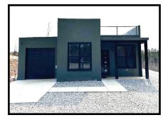
STORM RESISTANT HOUSING. Construction of storm resistant housing appears to be a growing trend nationally. EM Contingency Group of luka, owned by Mario & Elizabeth Barnes, has built a demonstration storm resistant house. Built of structural concrete insulated panels (SCIP), this construction method offers a storm resistant, low maintenance, energy-efficient home that is also fire and pest resistant. Designs are as flexible as traditional stick built homes.
